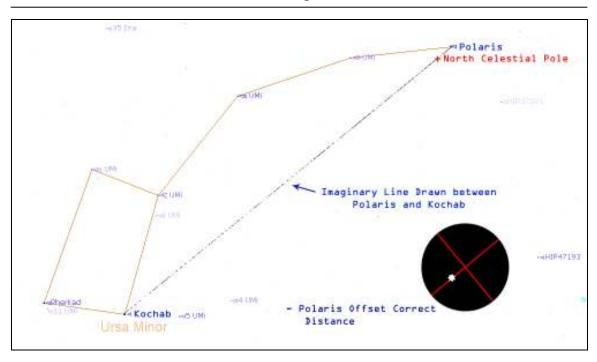
At this point, your telescope is probably within less then 5 arc seconds of the NCP and is ready for your normal alignment.
