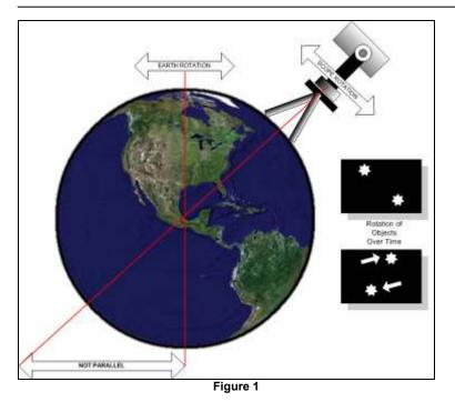
To alleviate this, telescopes can be mounted such that their center of rotation about the RA axis is parallel to the poles of the earth. As can be seen in Figure 2 below, the results of this are that only the RA axis must change its position over time. By matching the speed of the rotation of the earth and with the RA axis parallel to the poles of the earth, long exposure is made possible without the rotation that results from an Alt / Az setup.
