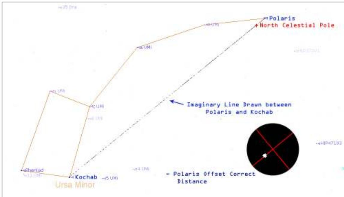
At this point, your telescope is probably within less than 5 arc seconds of the NCP and is ready for your normal alignment.
