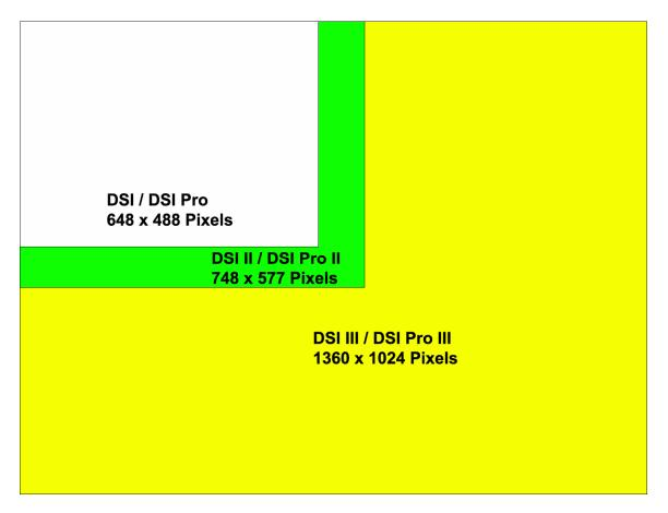
Of course, along with a larger image size comes a larger FOV. It should be noted that while the number of pixels is roughly double that of the DSI II, the pixels are smaller and as such, the FOV is not quite double that of the DSI II. However, as can be seen in the image on the following page, the FOV provided by the new chip is significantly larger then that provided previously and puts many larger objects on the chip in a single image that required a mosaic with the previous cameras.
