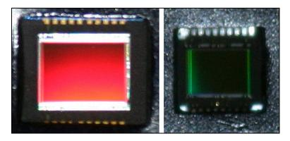
While the chip is larger then its previously used cousins, other major improvements not immediately noticed by just looking at the chip size are as a result of the pixel composition itself. The pixels in the DSI III cameras are 25% smaller then in previous versions with the pixels on these chips being 6.4 x 6.4 microns in size. This smaller pixel size greatly increases the capabilities of this camera for wide field DSO imaging
